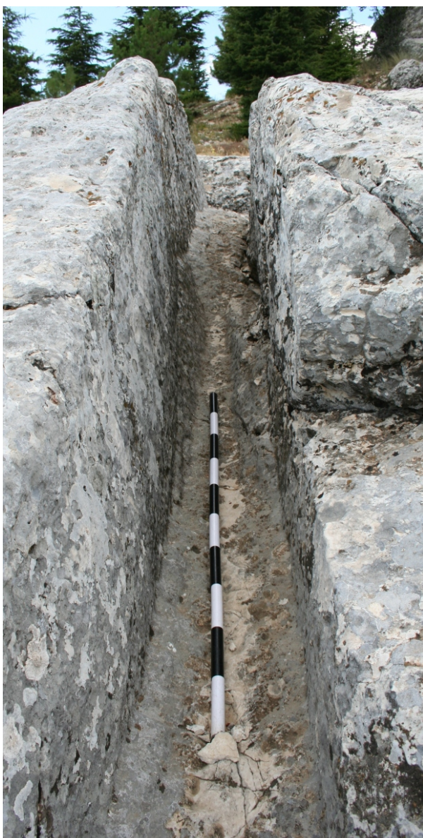
Carved channel in limestone for separating blocks from the bedrock
