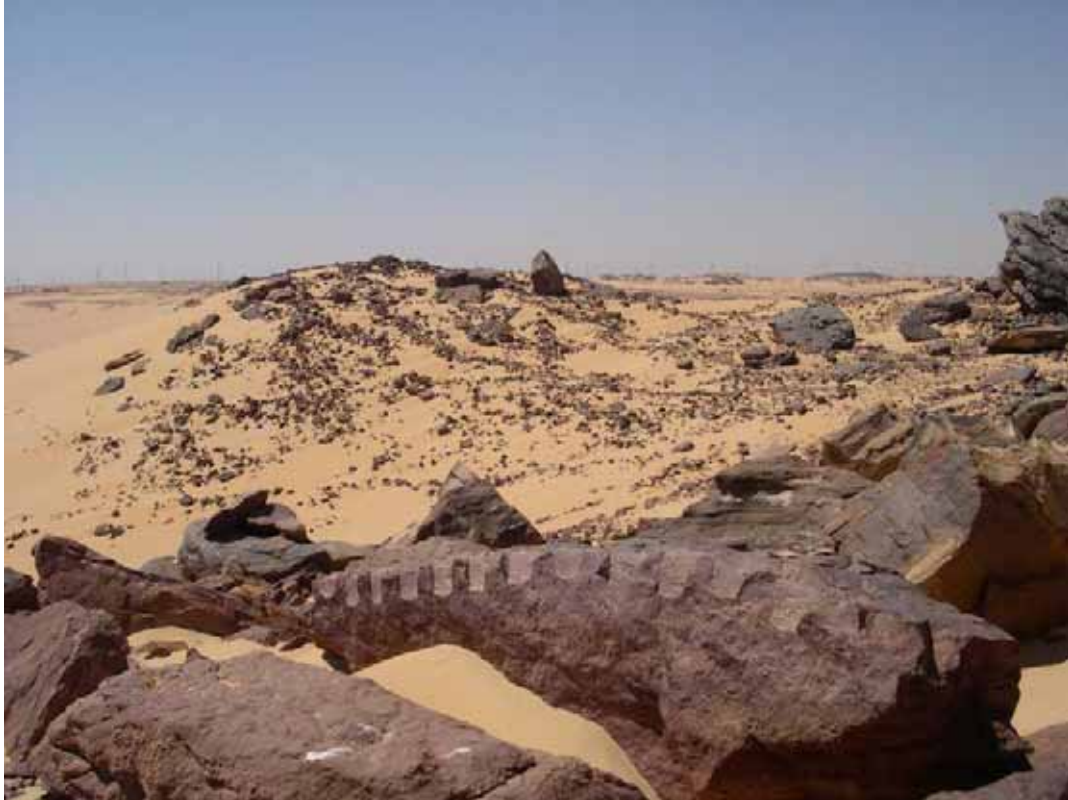
Roman wedge marks in a block of purple silicified sandstone, Gebel Tingar
